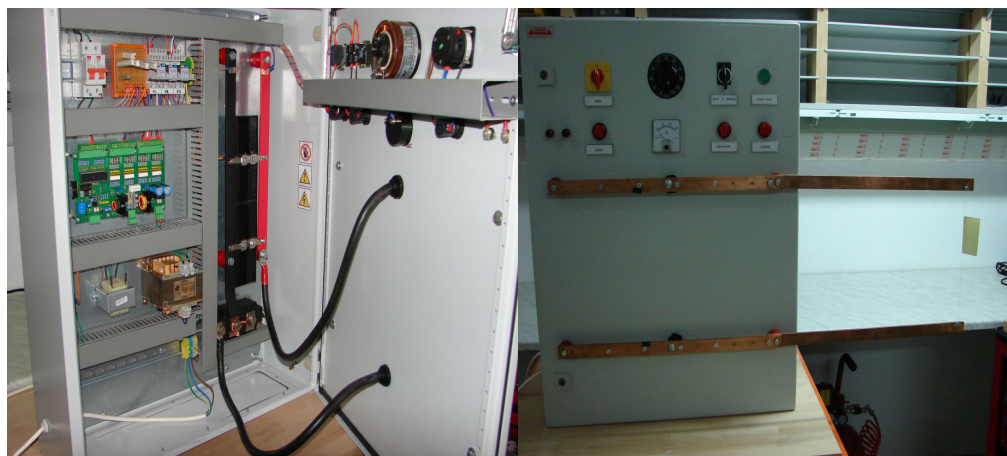
FIGURE 5. Exterior view of the whole device with the test wire attached (see white paper sign on the right)
